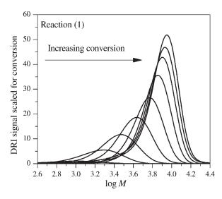
Molar mass distribution of samples scaled for conversion taken from reactions (1) where RAFT (1) was used, .All reactions conditions are listed in Table 1.
