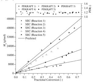
Figure 3. Evolution of  $\overline{M}_n$  and polydispersity as a function of conversion, for RAFT mediated polymerization of vinyl acetate prepared from reactions (1) to (5). Refer to Table 1 for reactions conditions.
